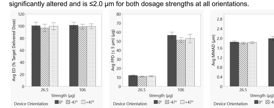
DUSA and APSD evaluations for 26.5 mcg and 106 mcg doses show dropping the DPI from 5 feet before or after puncturing the capsule has no significant effect on ED and FPD. APSD results for both doses show dropping the device does not significantly alter the MMAD.
